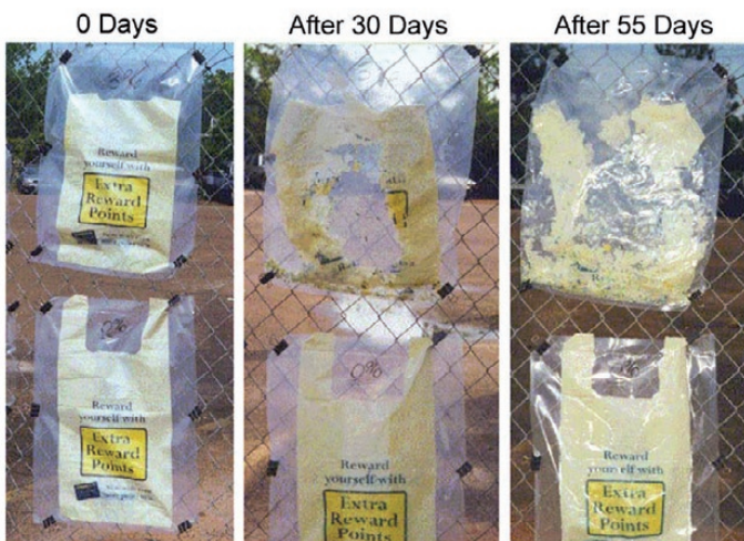
Illustration of photo and thermal degradation of a shopping bag incorporating EPI's TDPA® Additive (top row) vs. a bag without EPI's TDPA™ Additive (bottom row). Test procedures follow ASTM D5272 "Outdoor Exposure Testing of Photo Degradable Plastics" Guidelines.
